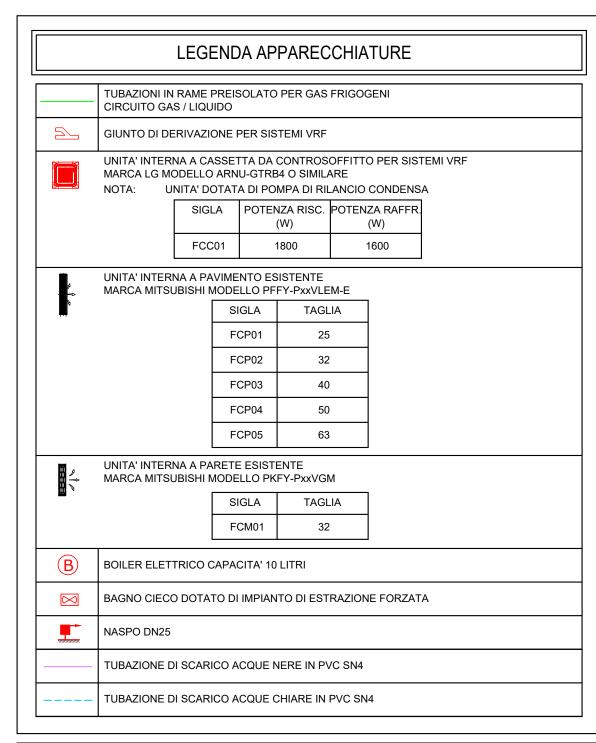
N.B.: LO SCARICO CONDENSA DI OGNI UNITA' INTERNA DOVRA' ESSERE DOTATO DI IDONEO SIFONE
